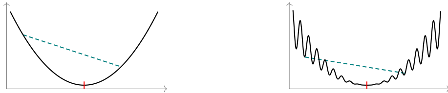
Figure 1: A convex (left) and non-convex (right) function. Both functions have their minimisers at the red mark. Only for the convex function (left) this minimiser can be determined by finding the stationary point. The non-convex function has several other stationary points. The teal dashed line illustrates the definition of convexity.
